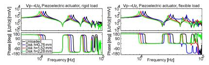
Figure 3: The influence of a rigid (left) and flexible (right) load on the dynamics of the vertical axis of a 60x10 mm (LxD) tube actuator.
