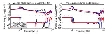
Figure 4: Modal actuation for varying load conditions by tuning in the in the case of an average disk thickness (1.52 mm) and by in-situ tuning (right).
