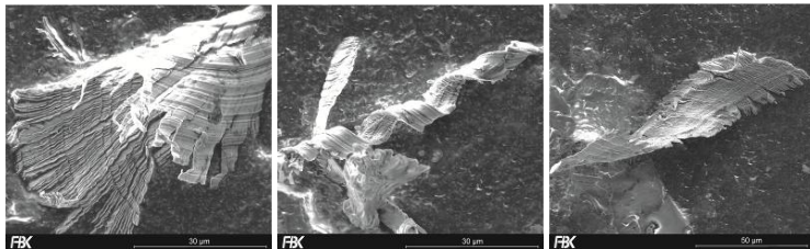
Figure 4: Chip types resulting of deep hole peck drilling process (after 4 holes)
