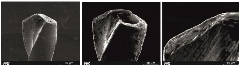
Figure 3: Used TiAlN-coated micro drill. From left to right: 4 holes and 24 holes and worn cutting edge
