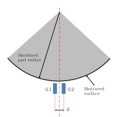
Figure 3. The measurement setup schematic for proposed two-probe differential method
