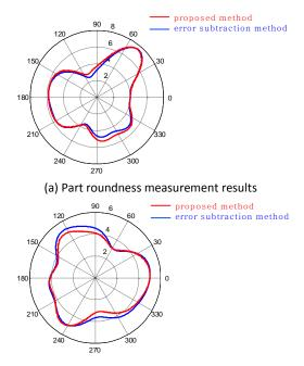
(b) Rotary table radial error motion measurement results
