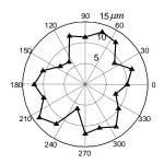
Figure 2. Roundness measurement result by the error subtraction method with dial gauges
