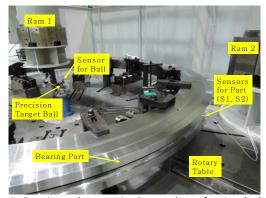
**Figure 4.** Experimental setup simultaneously performing both the proposed and the error subtraction methods using capacitive type displacement sensors
