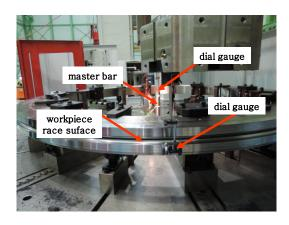
Figure 1. Previous experimental setup for the error subtraction method
