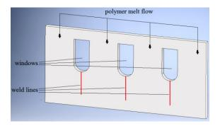
Figure 3. Expected weld lines in correspondence with the three windows
