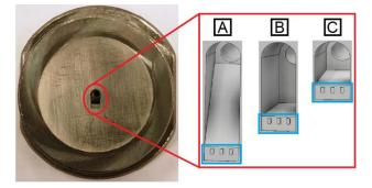
Figure 4. Changeable mould inserts with different runner and gates systems (A, B, C) for the simplified micro part (highlighted in blue)
