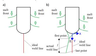
Figure 5: Formation of an ideal (a) and a possible actual (b) weld line
