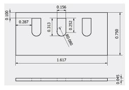
Figure 2. Simplified version of the real micro part containing the three windows (dimensions in mm)
