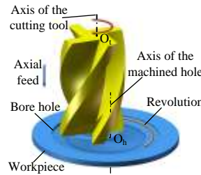
Figure 1. Schematic diagram of helical milling process
