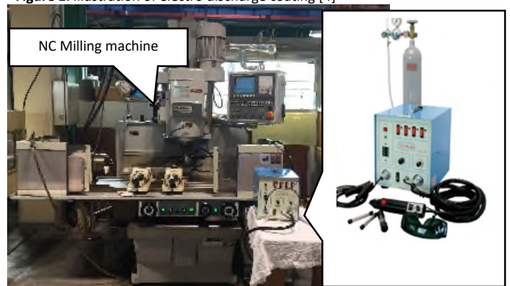
Figure 2. capacitor electro discharge deposition system (Micro depo) and how to set on milling machine [4]
