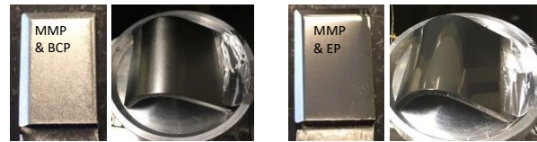
Figure 3. The comparison of the surface aspect of the niobium samples after MMP and BCP & EP.
