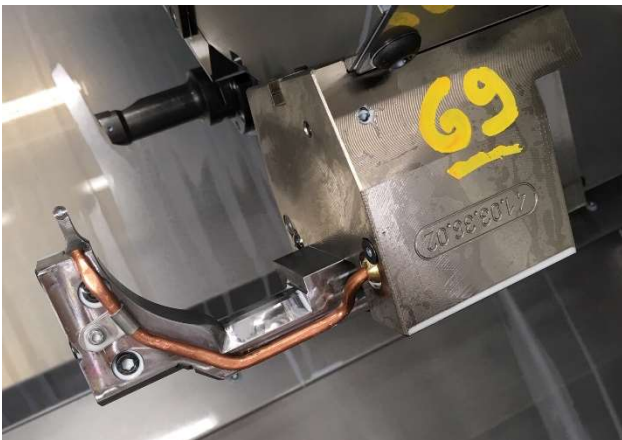
Figure 7. Final design of the toolholder mounted in the machine.
