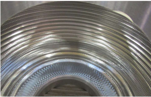
Figure 6. Inner cavity surface after roughing milling.
