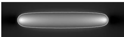
Figure 3 Section of a tomographed workpiece affected by beam hardening artifact
