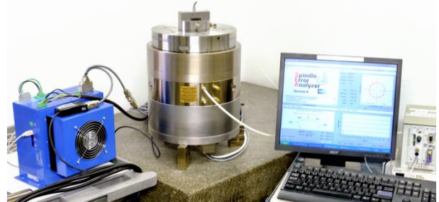
Figure 5. Test setup with motorized spindle, bespoke tooling, and data acquisition system. Low ball is 225 mm up from the spindle center.
