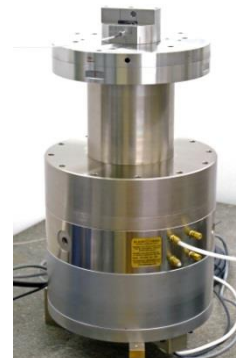
Figure 6. High ball test measuring radial errors 375 mm up from the center of the spindle.
