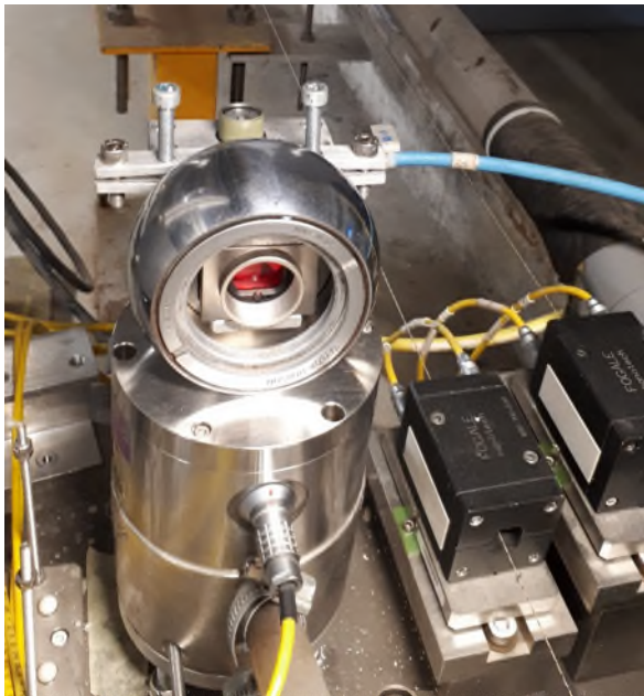
Figure 2. The camera mounted in the Taylor-Hobson ball adapter on the conical top of the HLS sensor (left) and the WPS sensor (right).
