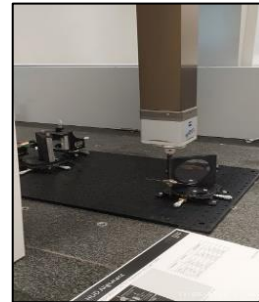
Figure 3. Coordinate metrology-based positioning and alignment of the freeform mirror-based HUD system.
