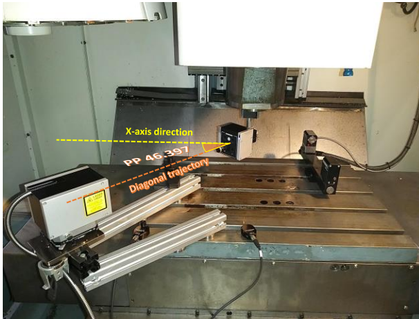
Figure 5. Experimental setup with Renishaw XM-60 laser system for face diagonal tests in XY plane of a VMC at PP 46.397 deg.
