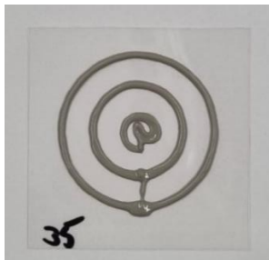
Figure 3. Adhesive applied to plastic sheet with the same pattern utilized in the aerostatic bearing manufacturing process.
