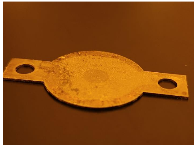
Figure 7. Test Sample After Photoresist Processing
