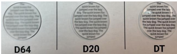
Figure 3. Visual comparison of ‘grayness’ of generated (D64 & D20) versus laser assisted diamond turned sample (right).
