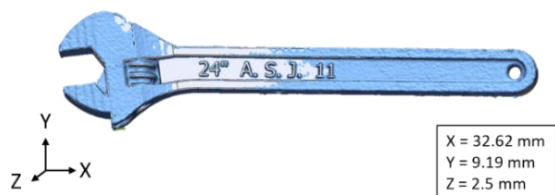
Figure 4. The scanned model in blue is superimposed on the reference CAD model in grey.
