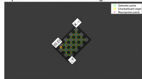
Figure 3. Detected points versus reprojected points from enhanced calibration using ABC.
