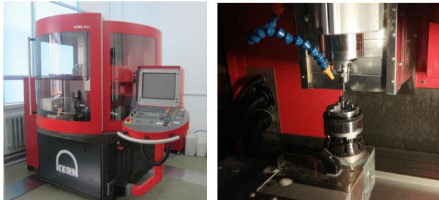
Figure 3: The 5-axis precision milling machine, KERN Evo
