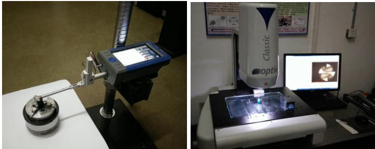
Figure 4: Workpiece detection and tool wear observation
