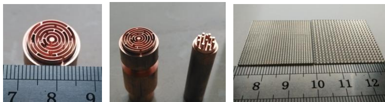
Figure 1: Some workpiece micromilled by the author
