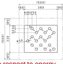
test pieces for punch presses and for laser cutting machines
