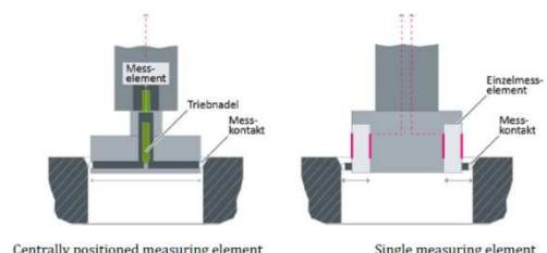
Centrally positioned measuring element
